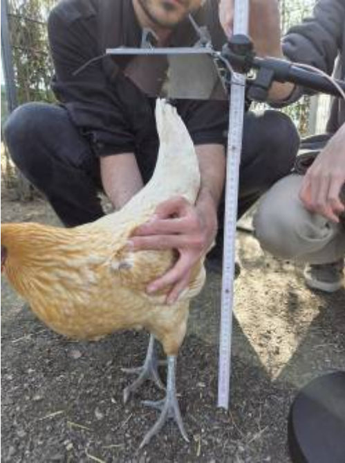
Approximate of 24 cm height of the rfid tag from the ground
