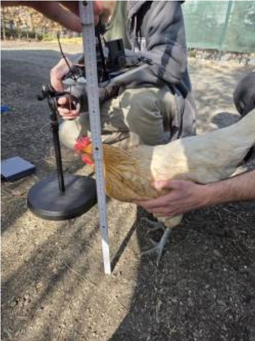
Antenna placed horizontally at 50 cm height on the ground able to read the rfid tag reliably. Antenna was then lifted up to at most 100 cm and still able to read the rfid tag (read range approximately 25-70cm).
