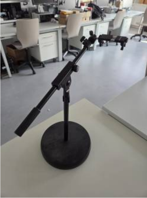
25 cm diameter for the base 44 cm height including base 44-74 cm for the arm
