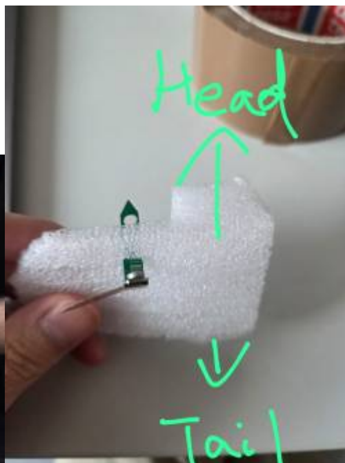
Tag is mounted from outer part of the wing to inner part as shown on the right. The rfid tag is faced
