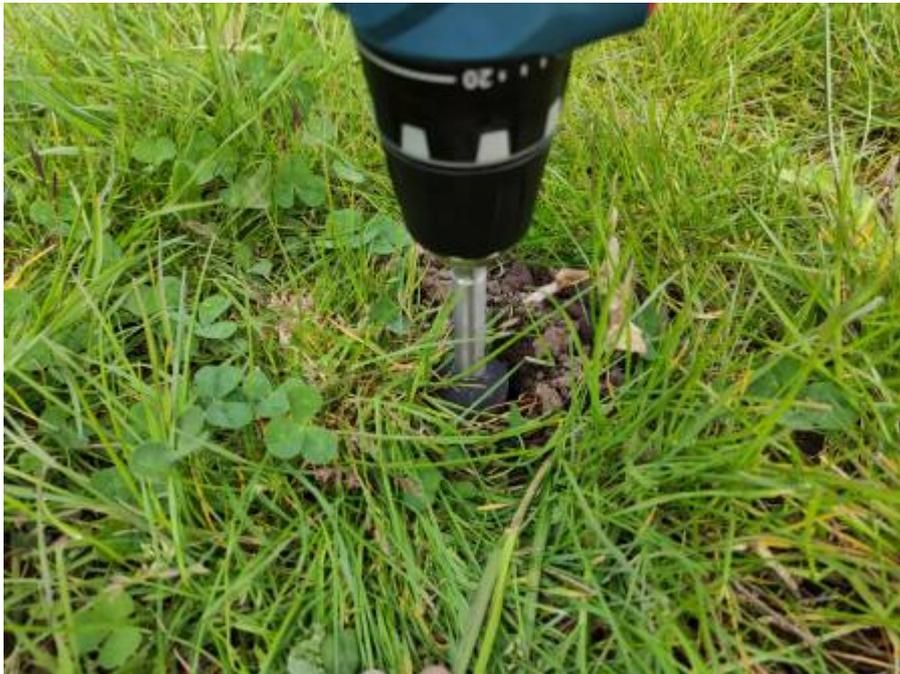
**Outlook:** From this test, I observed that it can not take the soil sample by drilling in one go, separate the total depth on multiple phases would be the best in this case. Measuring the torque in every moment, then when the torque demanded increases, finish that phase, clean the bit and continue with the next one.
