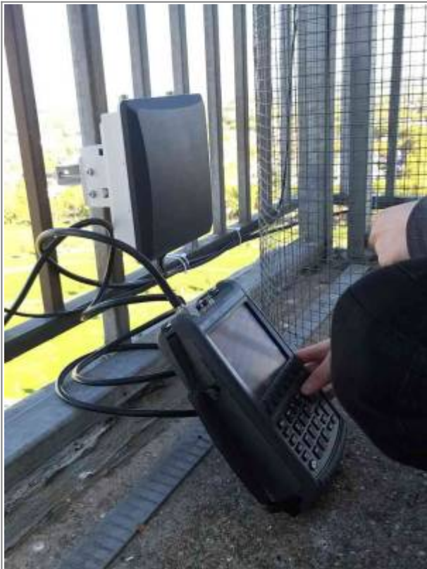
Fig.: Using a vector network analyzer to tune the antennne performance.
