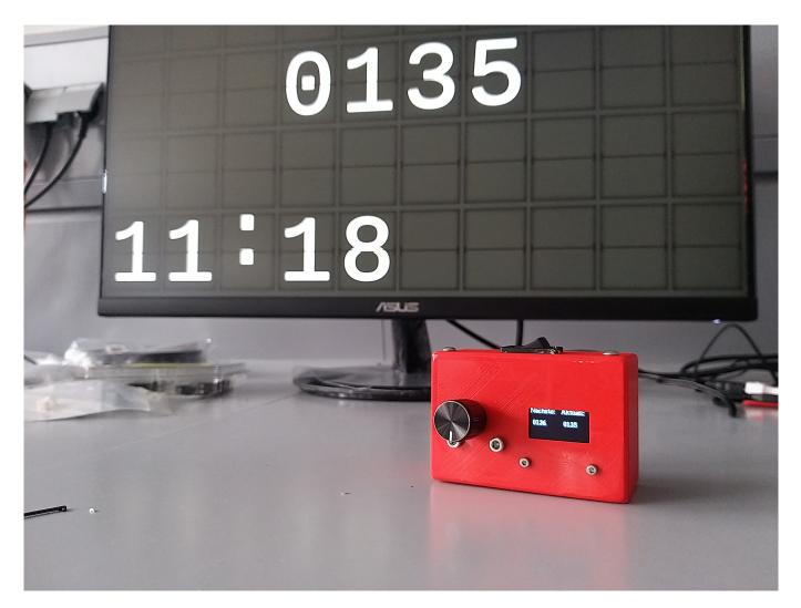
The controller consists of an ESP8266 with a battery, a rotary encoder, and a small display. All together in a 3d-printed housing. More information can be found here: Link to the Readme
