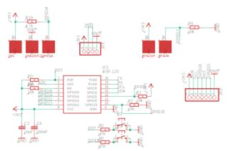
So a button press could be recognized as a rising edge. All other unused GPIOs (except GPIO2) are routed out to a little "development area". In this area, other sensors or daughter boards could be attached. Some examples can be found below in "Other possibilities".
