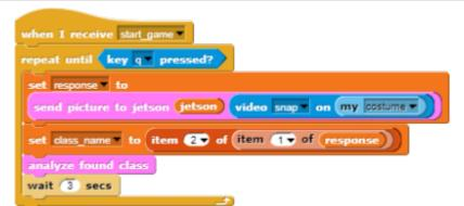
Inside **analyze** block we compare the class name with preset class names of food, that our pets consume, and broadcast to them. In case if the detected object is not suitable for any of them, we run **speak** block to pronounce the name of the object.
