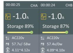
3) When the voltages of the two batteries are one higher and the other lower than the storage voltage, the high-voltage battery is discharged and stored, and the low-voltage battery is charged and stored, as shown in figure.
