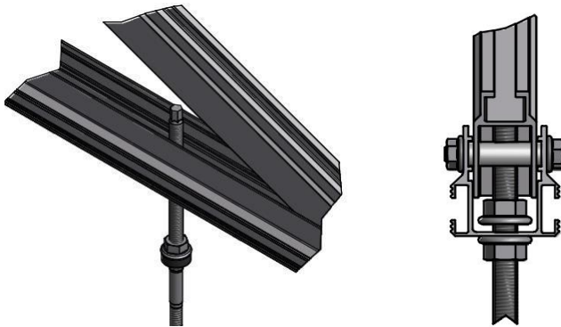
Figure 126: Fixation by hanger bolt
