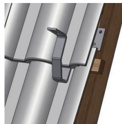
Figure 7: Fitted roof hook
