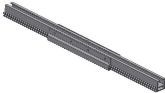
Figure 76: Joining together the carrier rails
