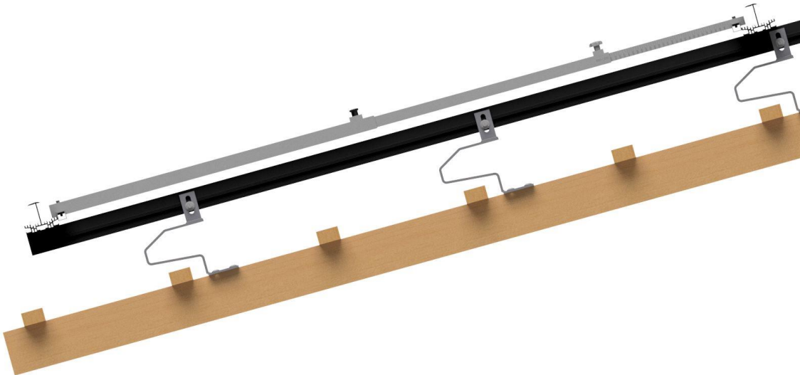
Figure 137: Positioned assembly jig
