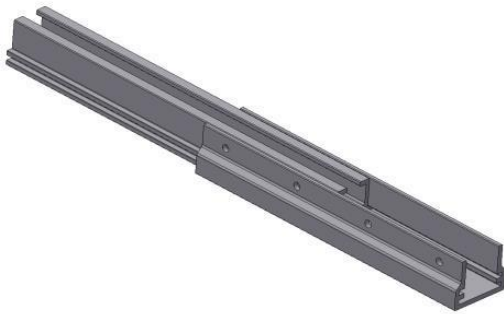
Figure 75: Insert butt connectors
